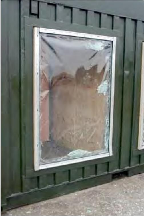
The test specimen lost approximately 94% of the glass from the outer surface of the film. The FrameGard Gullwing anchoring system became detached along a section of the left hand reveal measuring 380mm in overall length. The detachment of the anchoring profile allowed a small quantity of glass fragments to land inside the test cubicle. The total of the fragments weighed less than 50 grams.
