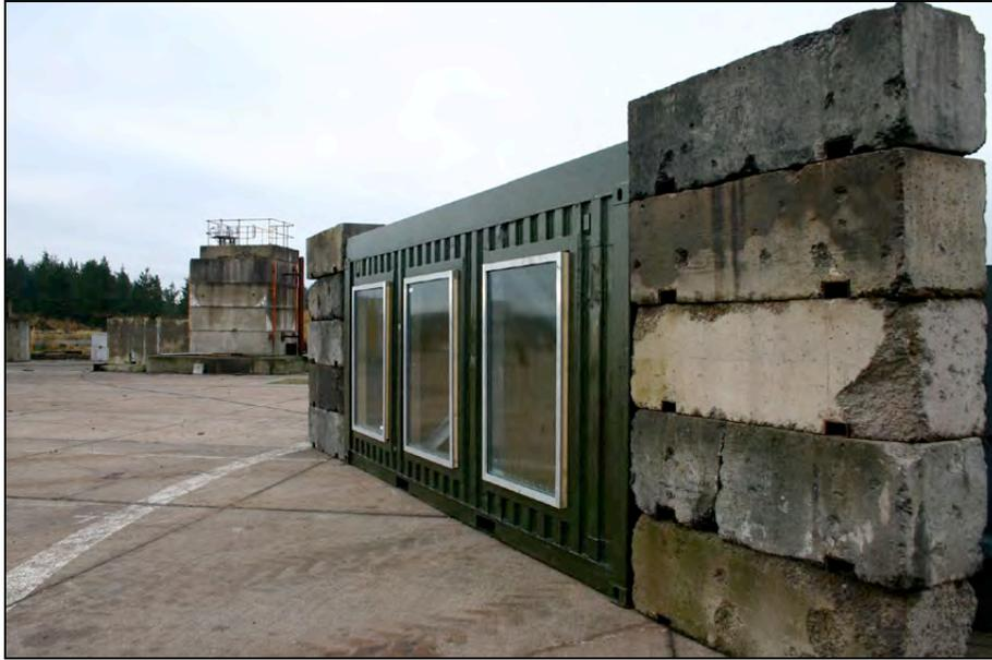
**P5: View of test structure prior to detonation**
