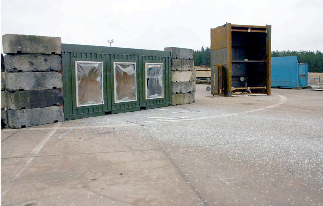
**P7: View of test cubicle post detonation of 100kg TNT at 31metres stand off.**
