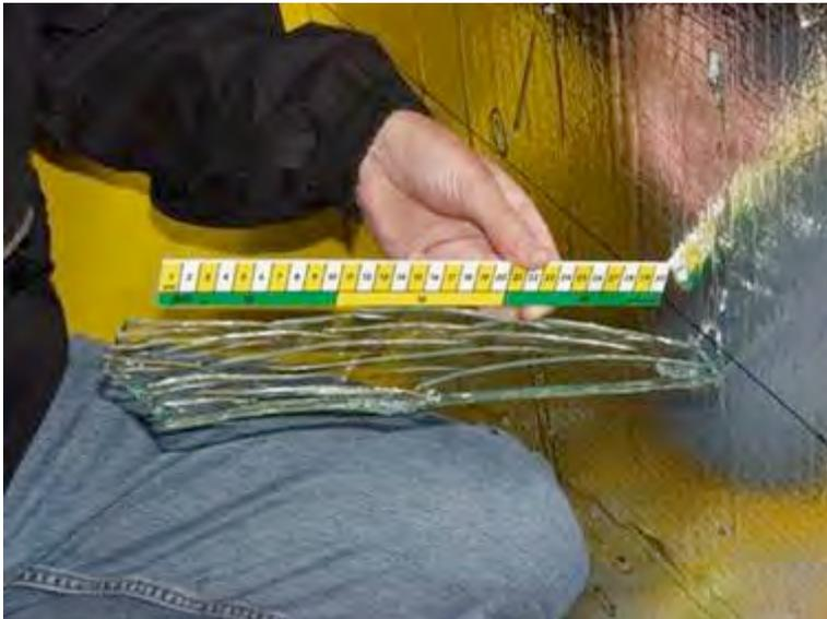
**P4:** Fragments of untreated glass measuring more than 300mm in length embedded into the rear witness panel.
