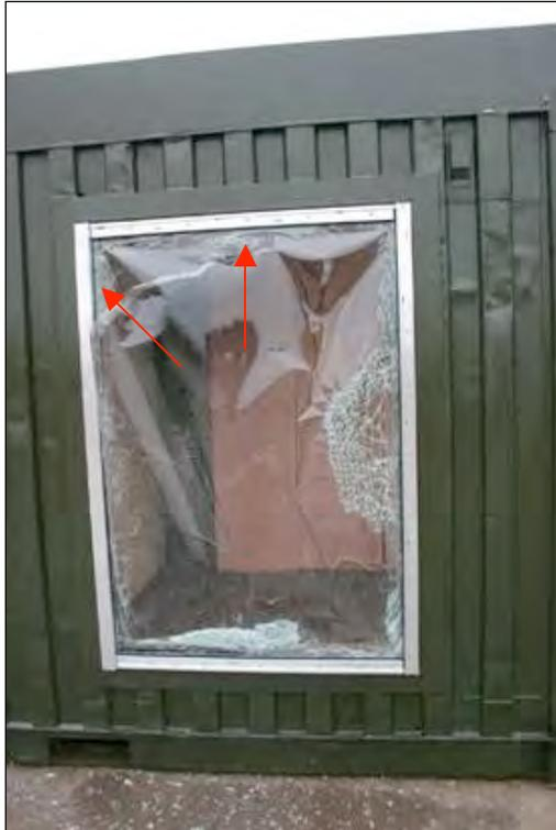
The FrameGard Gullwing anchoring system became detached along the left hand edge [in photo] and the window film split diagonally across over a length of 970mm at the position indicated by the arrows.
