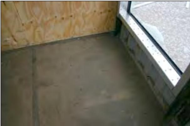
Glass fragments were discovered on the floor inside the test cubicle totalling less than 50 grams and thought to originate through a small edge tear in the window film. The fragments were all within one metre from the window.
