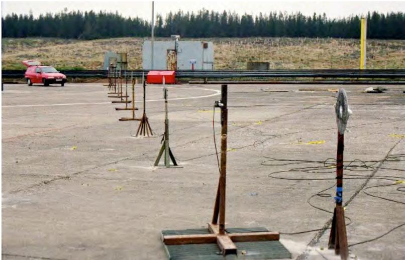
**P2: Free field gauges**
