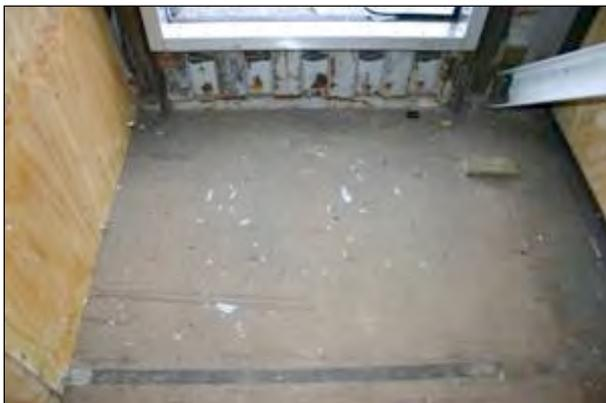
The glass scatter was primarily within the 3A Zone i.e. within one metre of the window sill.
