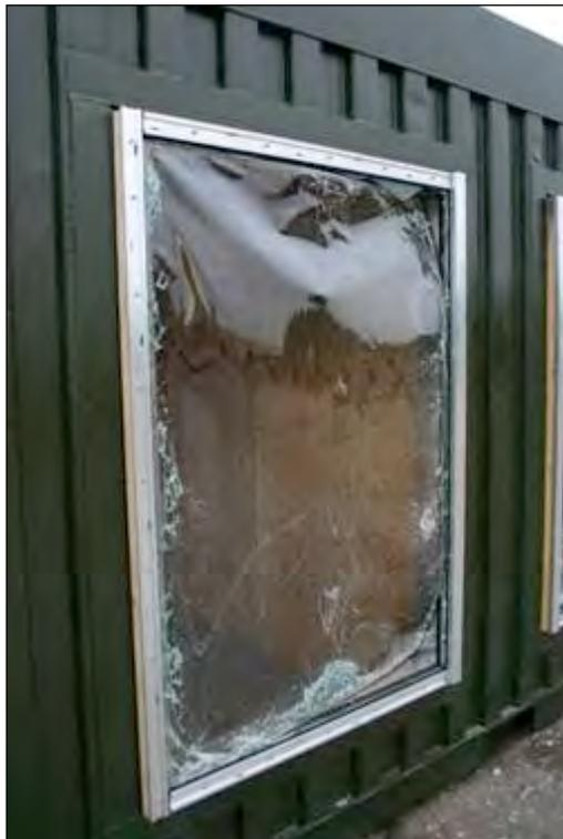
The test specimen lost approximately 92% of the glass from the outer surface of the film. The film split along the top right hand [880mm] and bottom right hand [989mm] corners.
